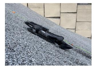
Figure 1. Picture of the Aliengo quadruped robot with novel, custom-designed torso (design 2) lying on a pile of pebbles with retracted legs.
