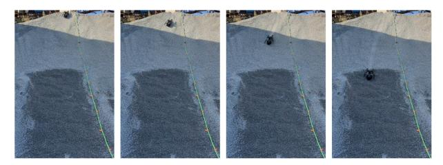
Figure 6. Image sequence of experimental trial of the Aliengo quadruped robot with custom-designed lower torso (version 2) sliding down an approximately 10m tall pile of pebbles without the need of swimming motion (from left to right, time between frames: 0.75s). The orange tape on the green rope is positioned every 1m and helps for a simple video analysis of the robot velocity.
