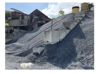
Figure 4. Picture of the field trial location close to IIT, in Genoa. The outdoor test campaign was performed on the 33° inclined pile of pebbles visible in the back.
